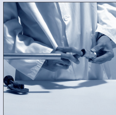
Fig. 23 Kontrol af O-ringens installation og placering Checking the presence and positioning of o-rings
